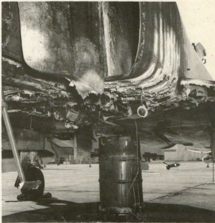
An unauthorized barrel, improperly grounded caused this static sparked fuel fire.
